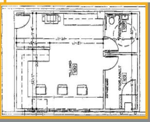
**Size/Availability:** The teller area is comprised of a 750 square feet and serves six motor bank lanes. One lane is served by a teller drawer, four lanes are served by tubes and one lane is set up as an ATM lane.
